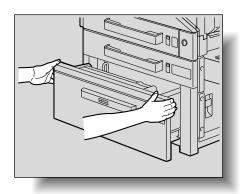
3 Load the paper into the right side of the paper drawer for the largecapacity paper feed cabinet so that the side of the paper to be printed on (the side facing up when the package was unwrapped) faces up.
